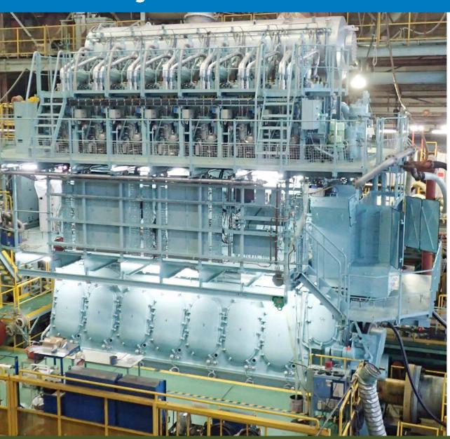
Kawasaki Heavy Industries, Ltd. completed of a Kawasaki-MAN B&W 7S60ME-C10.5-LGIP engine, an LPG-powered marine diesel engine to be used in a large LPG carrier being built at Sakaide Works for delivery to Kumiai Navigation (Pte) Ltd. This engine is the first MAN B&W S60 type LPG-powered engine to be produced in the world.
